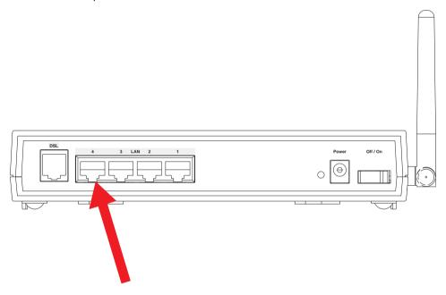
If you add devices connected through a hub or switch, connect the hub or switch to an Ethernet port on the Netopia 3347W/3357W-ENT.
